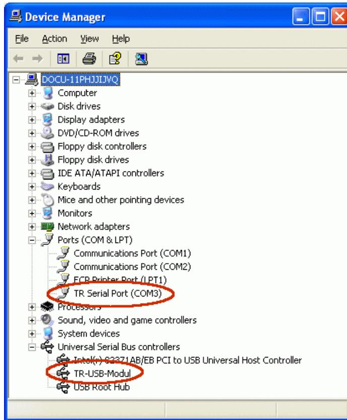
About the context menu (Right-click onto the entry) --> *Properties*, the Port number also can be changed. Only the port numbers COM1 ... COM9 are allowed!
