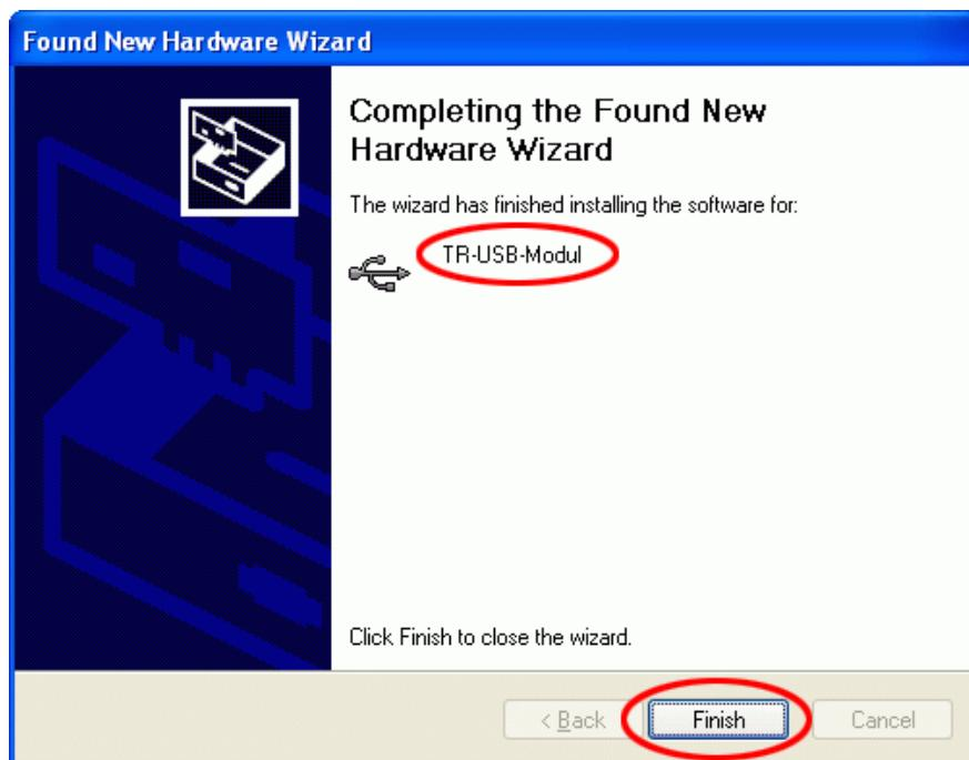
After this the *Found New Hardware Wizard* is started again for the **Serial Port**. If this is not the case, the driver software of COM port "TR-Serial-Adapter" must be installed manually again by means of the WINDOWS® device manager. The proceeding is the same as before. After finishing of the installation the PC adapter is functional.
