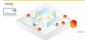
Holders of processing pallets are adjusted depending on a workpiece. The fieldbus control motors and encoders are used to adjust the holder as well as switches and solenoid valves for the cylinders.
