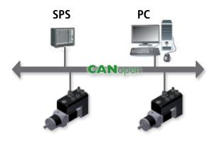
CANopen defines, for distributed industrial automation systems, a standardized protocol based on CAN. All common bit rates are accessible and set over a DIP-switch. The fast exchange of process data uses a process data object (PDO), the access to the entries within the object directory happens over service data object (SDO). All drive specific information is summed up within the object directory.
